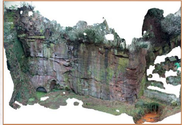
Photogrammetry and 3d laser scanning were used to record Worsley Delph in 2018. This is a 3d model that is made up of 70 photos taken from the ground
