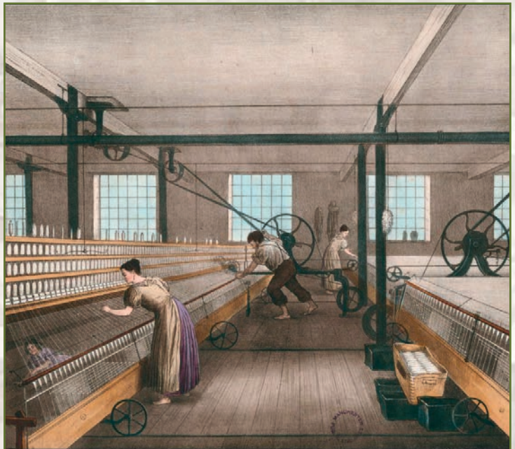
Spinning mules captured on a coloured lithograph by James Barfoot in 1840. Note the child collecting cotton waste beneath the moving machinery
