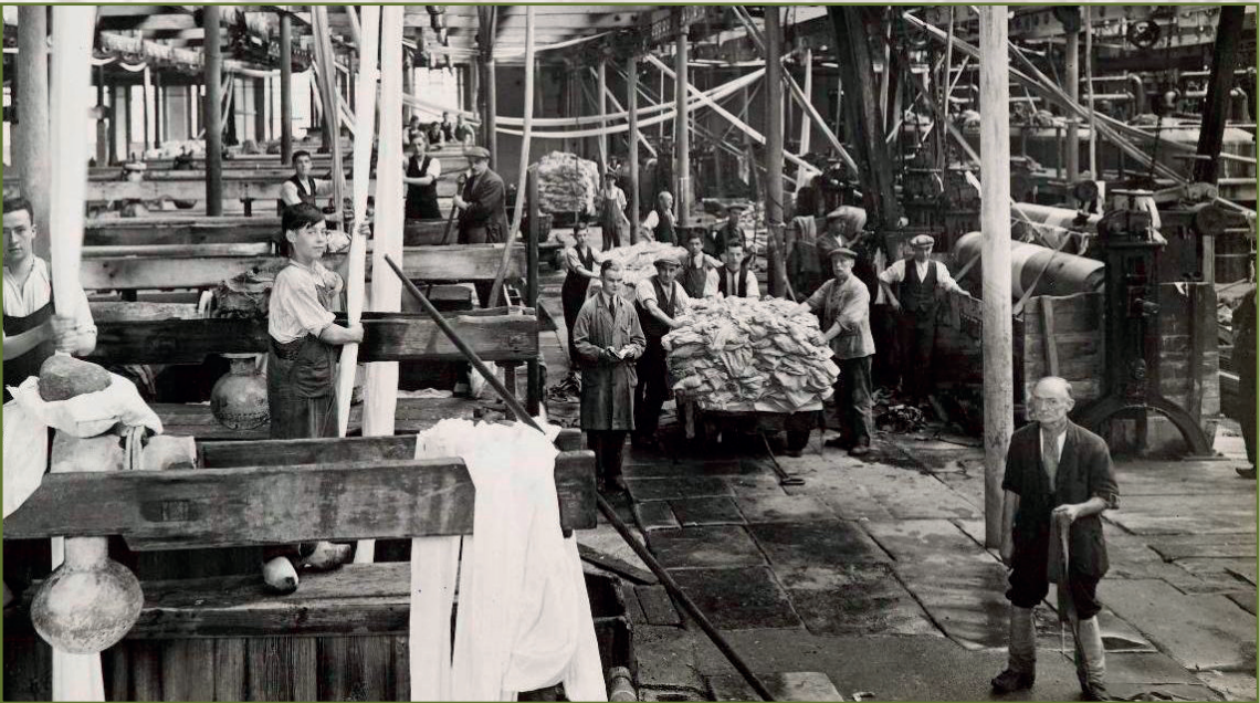
The interior for a bleach croft in the early 20th century, showing the rope of cloth passing between the different stages in the bleaching process
